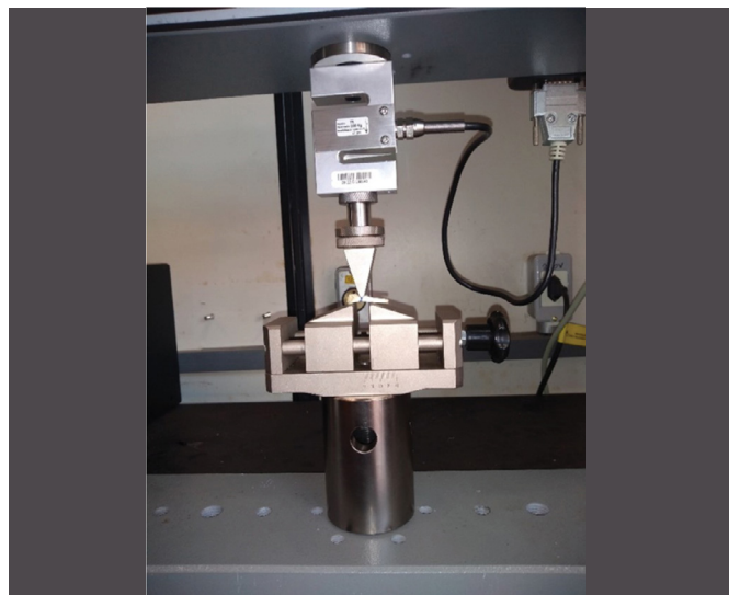
Figure 1. Experimental setup for the three-point bending test of the rat tibia.
