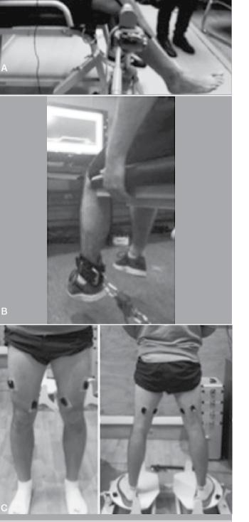
**Figure 1.** (A) Shows the joint position sense test with the uniaxial electrogoniometer. (B) Shows the steadiness test with the load cell and the paradigm to 15% of the MVIC. (C) Shows the knee muscle onset test with the position of the sEMG sensors and the platform.
