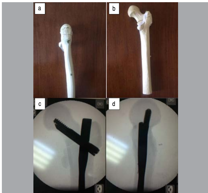
Figure 1. A and B: fracture model fixed with antirotator proximal femoral nail; C and D: fixation under image intensifier.
