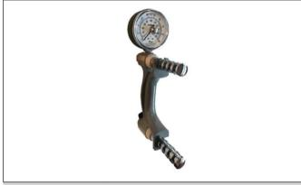
Figure 3. Manual pressure dynamometer used in the tests.
